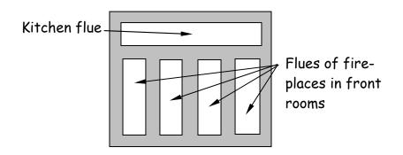
Exposed to the sky, these open flues absorb a great deal of water. When the chimney is inactive, as at the parsonage, this moisture saturates much of the masonry. The only means by which the chimney rids itself of the water is through evaporation in warm, dry weather. This evaporation is aided by convection currents that naturally rise through the chimney flues and help to carry off the moisture.
