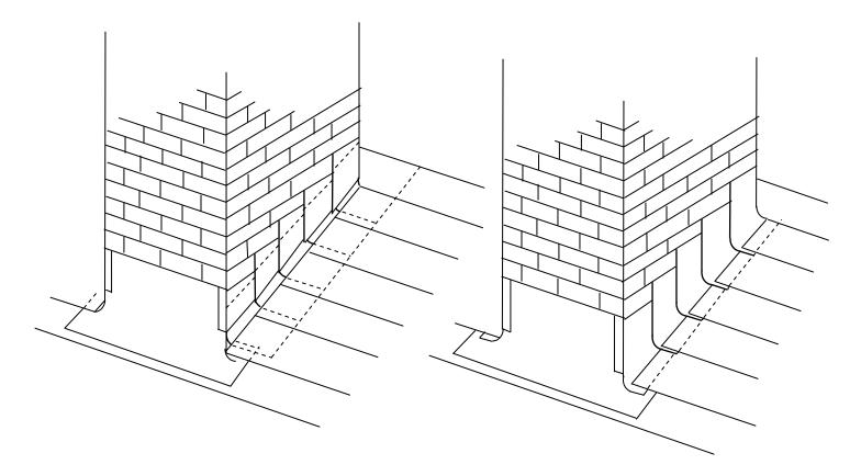
Cap and base flashing The best practice Flashing tucked under shingles Common but poor practice
