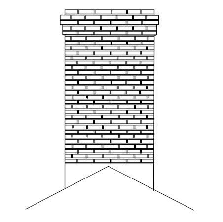
Typical chimney cap: two courses corbeled out about  $\frac{1}{2}$  inch, two more courses corbeled out  $\frac{1}{2}$  inch beyond that, and one cap course brought back into alignment with the main stack, usually covered with a "wash" of mortar or cement to shed water.
