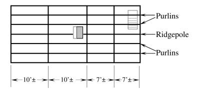
Trenches in the tops of the southern gable rafters may have been intended either for purlins extending over a now-missing bay of the frame, or for lookouts to support an overhang of now-missing raking eaves. The former seems more likely. This suggests that the frame was originally longer than its present length of approximately thirty-four feet, but that it was shortened by one or more bays when being converted to a dwelling or when being moved across the road from its original location.
